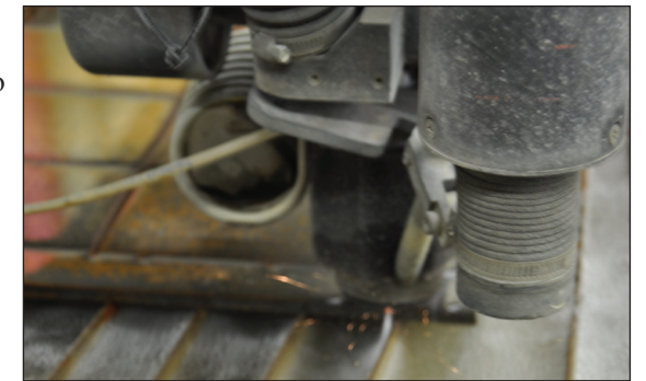
One of three water jet machines on Production Plant Barstow, Marine Depot Maintenance Command, cuts through metal using high pressured water and garnet, June 17. The water comes out at pressures up to 90,000 pounds per square inch, causing sparks to fly when it hits the metal.
