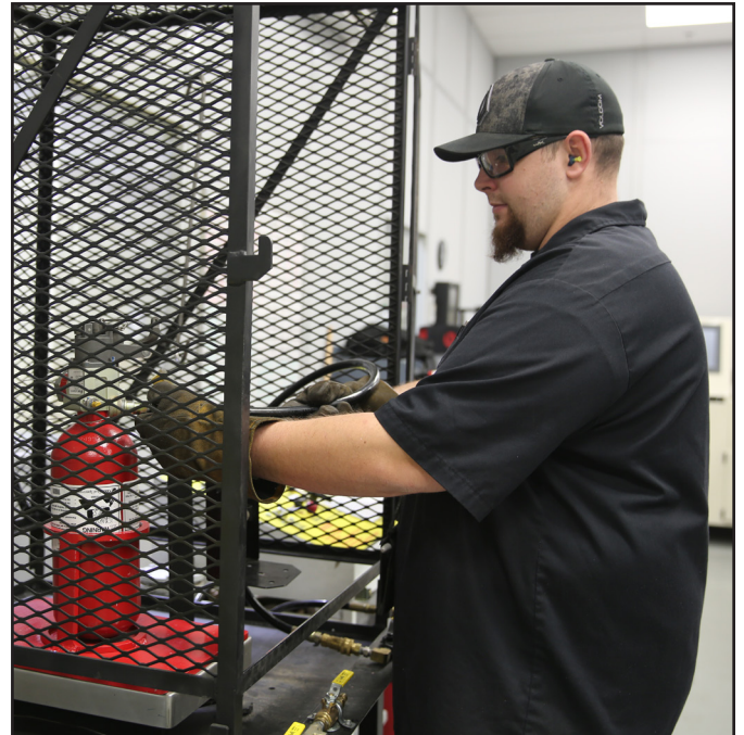
Luke Wirick, a hydraulics systems mechanic with the hydraulic shop on Production Plant Barstow, Marine Depot Maintenance Command, on Marine Corps Logistics Base Barstow, Calif., charges a light armored vehicle's fire bottle, Nov. 24.
