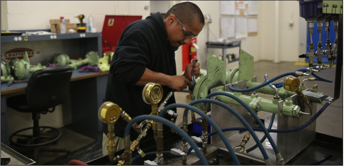
Cesar Meneses, a contractor with the hydraulic shop on Production Plant Barstow, Marine Depot Maintenance Command, on Marine Corps Logistics Base Barstow, Calif., Yermo Annex, tests a brake booster for a light armored vehicle, Nov. 24.
