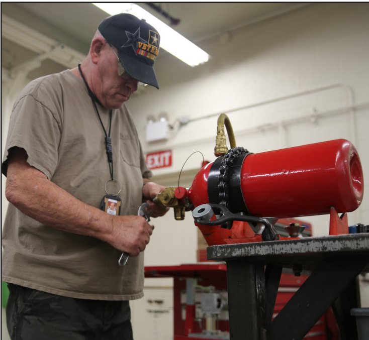
John Alley, a hydraulics systems mechanic with the hydraulic shop on Production Plant Barstow, Marine Depot Maintenance Command, on Marine Corps Logistics Base Barstow, Calif., assembles a 17-pound fire bottle for the light armored vehicle, Nov. 24.
